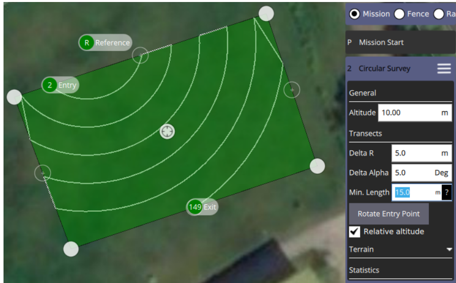
Figure 11: An example of a Circular Survey pattern.
