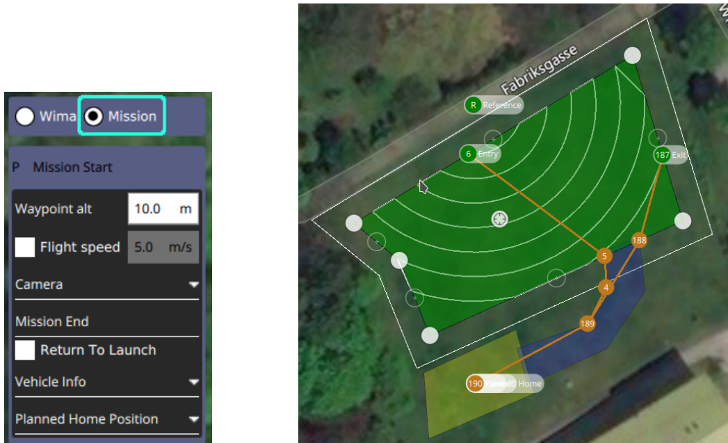
(a) Checking the Mission radio button, (b) The flight path generated from the areas depicted in fig. 10a. on the right hand side, displays the mission items.
