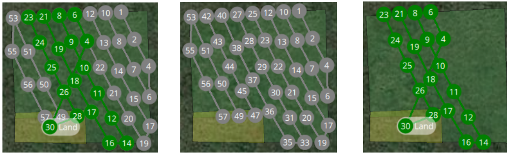
(a) Mission items (gray) and current phase (green) overlaid. (b) Mission items only (Show Phase unchecked). (c) Current phase only (Show Mission unchecked).
